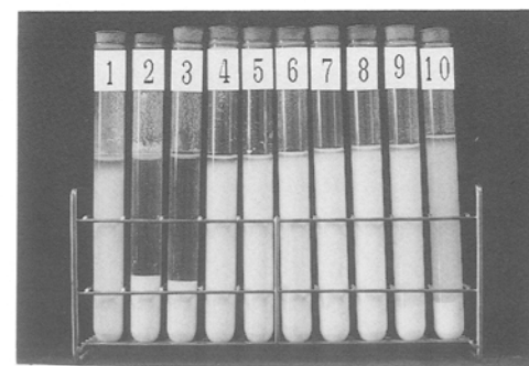
Figure 2 Sedimentation tests of (a) monoclinic and (b) tetragonal zirconia particles in aqueous suspensions in the presence of PAA. The amounts of PAA (wt % to ZrO_2 ) are (1) no addition, (2) 0.25, (3) 0.5, (4) 1, (5) 2.5, (6) 5, (7) 8, (8) 10, (9) 15 and (10) 25.
